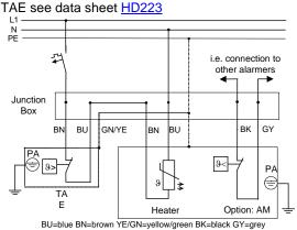
Connection cable Silflex-EWKF 3 x 1.5 mm<sup>2</sup>, 1m long. Other lengths available upon request (at an extra charge).
