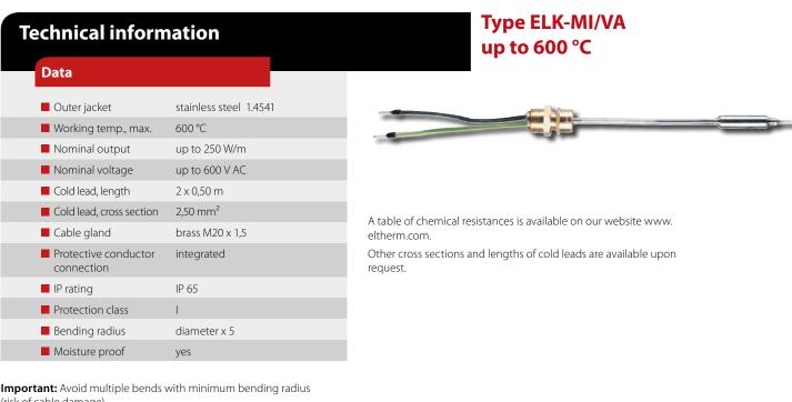
Important: Avoid multiple bends with minimum bending radius (risk of cable damage).
